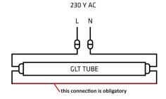
Picture 2: Electrical diagram multi-lamp
